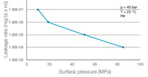
The graph shows the required stress at assembling to seal a certain tightness class. The determination of the graph is based on EN13555 test procedure which applies 40bar Helium at room temperature. The sloping curve indicates the ability of the gasket to increase tightness with raising gasket stress.
