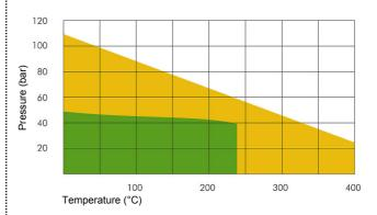
The P x T diagram above indicates the service limits for **NA-1005** considering the simultaneous influence of pressure and temperature (chemical suitability assumed). The green area represents the normal service limits, while the orange colored area shows the maximum application limits. For those cases, please consult our technical department.
