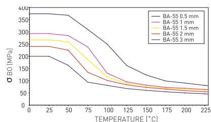
$\sigma_{BO}$  diagram represents  $\sigma_{BO}$  values for different gasket material thicknesses. These values indicate the maximum in-service compressive pressures which can be applied on the gasket area involved without destroying or damaging the gasket material.
