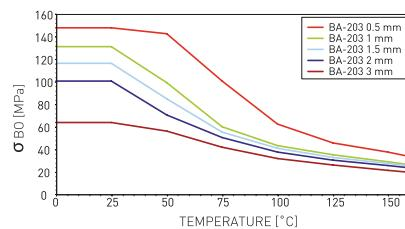
σ<sub>BO</sub> diagram represents σ<sub>BO</sub> values for different gasket material thicknesses. These values indicate the maximum in-service compressive pressures which can be applied on the gasket area involved without destroying or damaging the gasket material.
