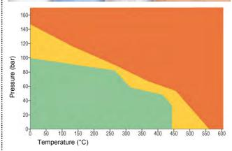
The P x T diagram above indicates the service limits for **NA-1122** considering the simultaneous influence of pressure and temperature (chemical suitability assumed). The green area represents the normal service limits, for the yellow area consultation is recommended, while the orange coloured area shows the maximum application limits for which technical consultation is mandatory.
